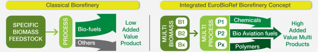
The EuroBioRef basic concept uses a new flexible approach to combine "virtual integration" with proximity to both feedstock sources and product markets:
